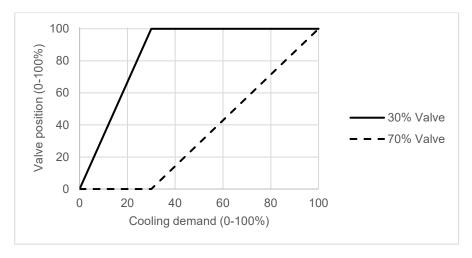
The object of this operating strategy is to achieve the maximum amount of cooling required for the minimum amount of the coil cooling capacity available. This will also de-humidify the air and provide the potential to maintain comfort levels while allowing the temperature set point to be raised, with a consequent saving in energy.
