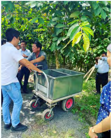
The stainless-steel in-field washing unit—designed through the ACIAR project—now widely used by growers to improve fruit quality and reduce post-harvest losses.
