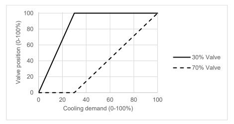
The object of this operating strategy is to achieve the maximum amount of cooling required for the minimum amount of the coil cooling capacity available. This will also de-humidify the air and provide the potential to maintain comfort levels while allowing the temperature set point to be raised, with a consequent saving in energy.
