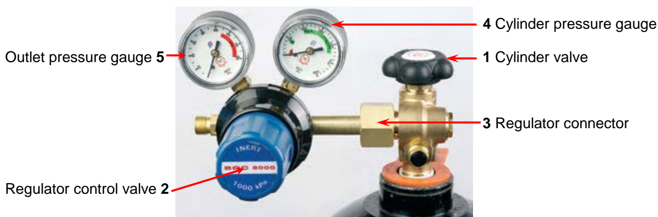
Figure 1 Typical side entry attached regulator (non-flammable gas).
