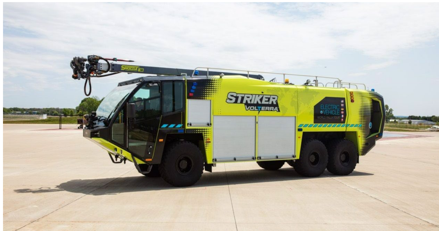
Striker Volterra 6x6 is a Plug-in Hybrid-Electric (PHEV) ARFF vehicle
