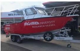
RV Medusa Class 2C 7.0m Half-cabin vessel 6-person capacity 2 x 135hp outboards
