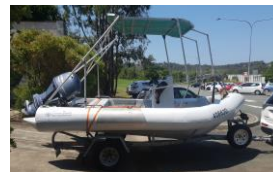
RV Rachel Carson Class 2D 4.65m Polyethylene centre-console 4-person capacity 60hp outboard
