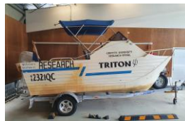
RV Triton Class C 4.7m Dual-hulled work boat 5-person capacity 80hp outboard
