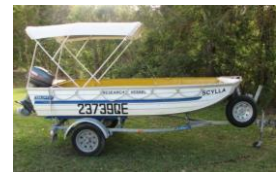
RV Scylla Class 2E 3.75m Aluminium dingy 4-person capacity 15hp outboard
