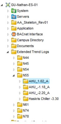
Extended trend logs are the connection used for data transfer to the historian and maintaining the first portion of the name (or placing in folder) as the Asset\_ID approach will significantly reduce the work of passing data between systems.
