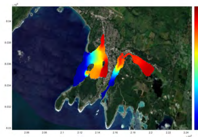
Model outputs of time to flush pollutants within Erakor Lagoon
