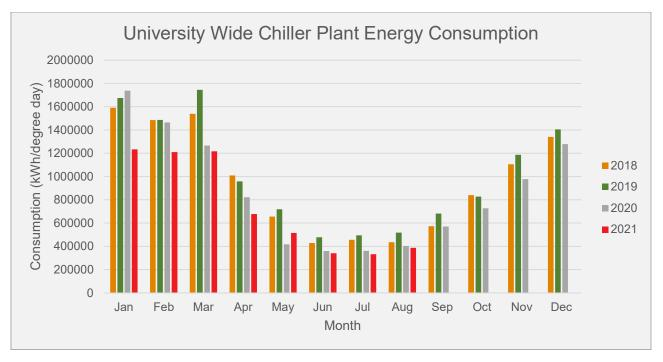
A significant contributor to the reduction in energy consumption was the relatively cool summer in 2021. To factor out the impact of the cooler summer, a ratio of monthly chiller plant energy consumption to *cooling degree days* was calculated for the months of November to March and is shown in the graph below. *Cooling degree days* is a commonly used measure for estimating how much air conditioning energy is needed for a period based on the outside air temperature curve.
