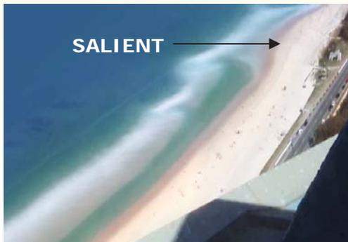
Extensive digital imagery, hydrographic survey and observational monitoring tells us that beach widening has been achieved. Since construction, the beach at Narrowneck has widened by about 40 metres, and maintained this width for over a decade (Figures 4 and 5).
