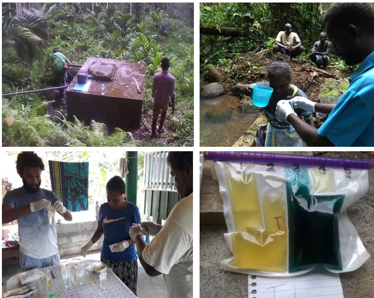
Figure 2.8: Water quality testing and site risk assessment activities (Green liquid indicates presence of E. coli ) (Photo credit: D Gonzalez-Botero, C Beal and M Love)
