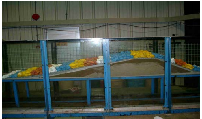
Figure 4. The view of the breakwater after completion of the construction
