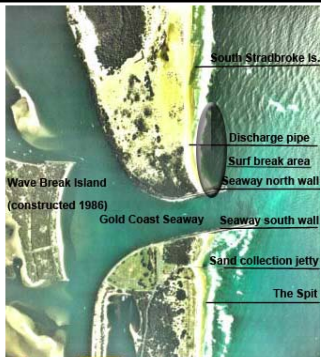
Figure 2. Photo of the Gold Coast Seaway and South Stradbroke Island. Source: Adapted from POUND (2002) for this paper.
