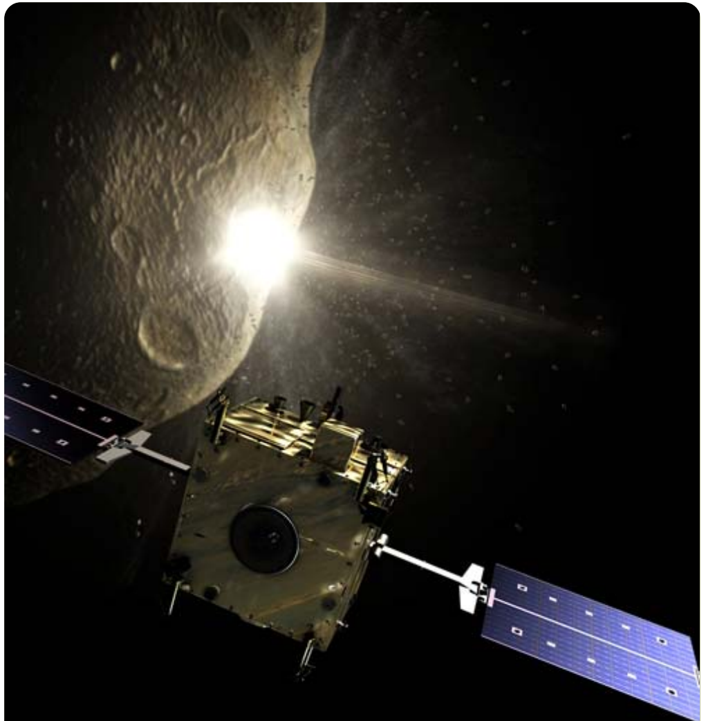
This simulated image shows the orbiter craft Sancho observing the impactor craft Hidalgo slamming into an asteroid to alter its trajectory.
